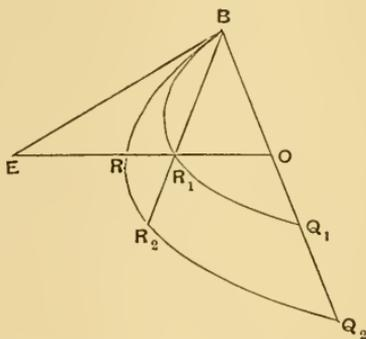
Suppose the problem solved, and let  $ERR_1O$ , parallel to the axes, meet the parabolas in  $R, R_1$  and  $BQ_2$  in  $O$ , making the intercept  $RR_1$  equal to  $l$ .
