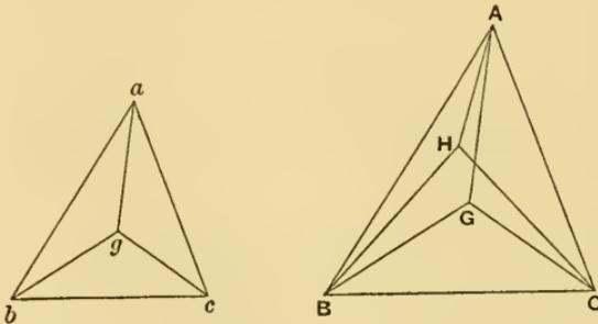
The proposition is proved by an obvious *reductio ad absurdum*. For, if  $G$  be not the centre of gravity of the triangle  $ABC$ , suppose  $H$  to be its centre of gravity.
