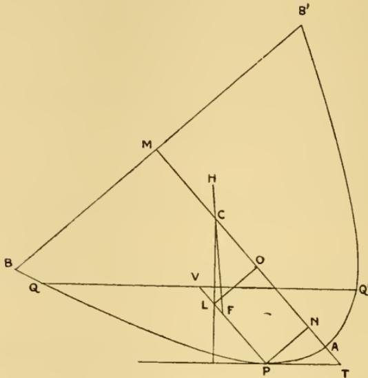
Let the plane through  $AM$  perpendicular to the surface of the fluid cut the paraboloid in the parabola  $BAB'$  and the plane of the surface of the fluid in  $QQ'$ . Let  $PT$  be the tangent parallel to  $QQ'$ ,  $PV$  the diameter bisecting  $QQ'$ . Divide  $AM$  at  $C, O$  as before, and draw  $OL$  perpendicular to  $PV$ .
