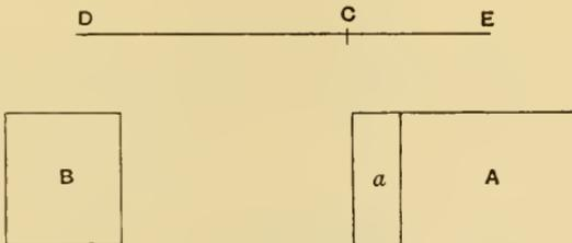
Then, if  $(A + a)$  placed at  $E$  and  $B$  placed at  $D$  do not balance about  $C$ ,  $(A + a)$  is either too great to balance  $B$ , or not great enough.
