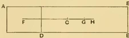
For, if the centre of gravity of the remainder ( $DE$ ) be not  $G$ , let it be a point  $H$ . Then an absurdity follows at once from Props. 6, 7.
