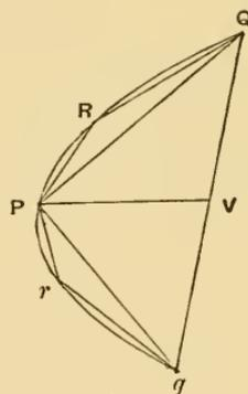
If then we inscribe in the segments cut off by  $PQ, Pq$  triangles which have the same base and equal height, i.e. triangles with the same vertices  $R, r$  as those of the segments, and if in the remaining segments we inscribe triangles in the same manner, and so on, we shall finally have segments remaining whose sum is less than the area by which the segment  $PQq$  exceeds  $K$ .
