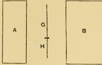
Let  $A$  and  $B$  be now combined into one solid and immersed. Then, since  $(A + B)$  will be of the same weight as the same volume of fluid, both weights being equal to  $(G + H) + G$ , it follows that  $(A + B)$  will remain stationary in the fluid.
