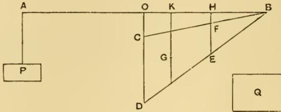
Draw  $KG$  parallel to  $OD$ , and let  $G$  be the middle point of the portion of  $KG$  intercepted within the trapezium. Then  $G$  is the centre of gravity of the trapezium [*On the equilibrium of planes*, I. 15].
