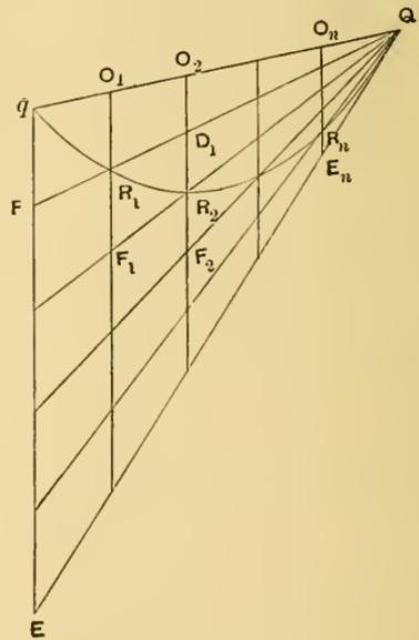
Let the triangle  $FqQ$  be such a submultiple of the triangle  $EqQ$ . Divide  $Eq$  into equal parts each equal to  $qF$ , and let all the points of division including  $F$  be joined to  $Q$  meeting the parabola in  $R_1, R_2, \dots R_n$  respectively.
