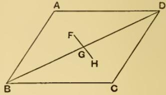
But [by *Post. 4*]  $F$  will fall on the centre of gravity of  $CDB$ . Therefore  $H$  is the centre of gravity of  $CDB$ .
