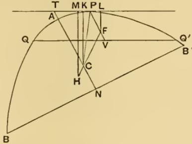
Then, since  $AN$ , as placed, is not perpendicular to the surface of the fluid,  $QQ'$  and  $BB'$  will not be parallel.
