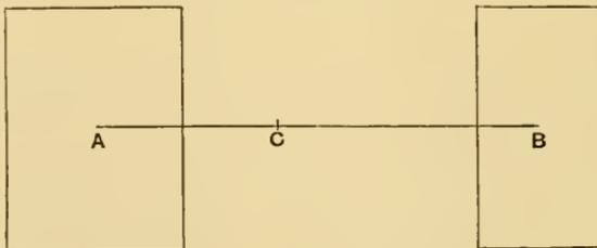
Then shall  $AC$  be less than  $BC$ . For, if not, take away from  $A$  the weight  $(A - B)$ . The remainders will then incline
